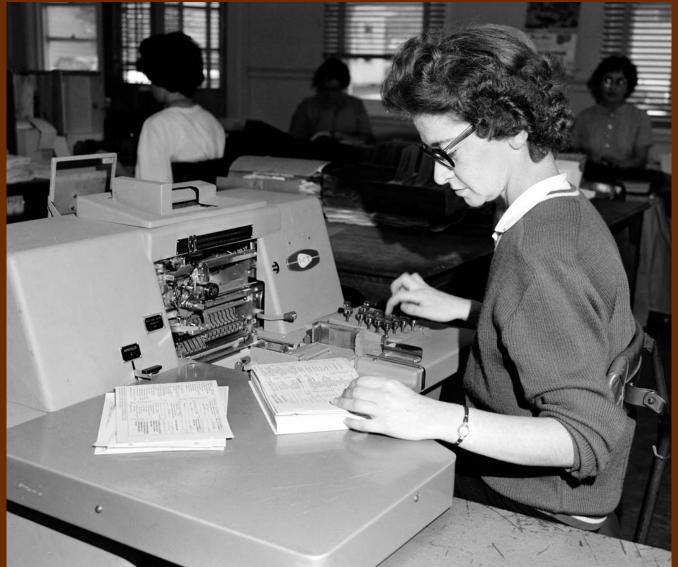
Operator of an ICT electric punch machine inputting respondent data from cards used in the labour force survey in the 1960s.
