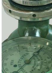
A Mullen Burst Testing machine, patent 1909, used to measure how much pressure could be applied to fabric before it burst. This is still used as a measure of fabric quality.
