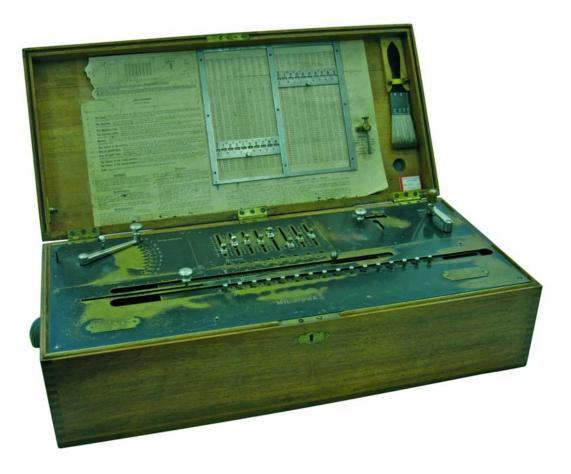
at an experimental stage and would have required considerable modifications to be suitable for Australia. However, Burroughs' Adding Machines were used for tabulations by locality and a Millionar calculating machine was also used. Unlike other adding machines of the period, the Millionar could do multiplication. The Millionar involved relatively new technology and this machine was one of only a couple of thousand in the world at that time. Above: The Millionar calculating machine.
