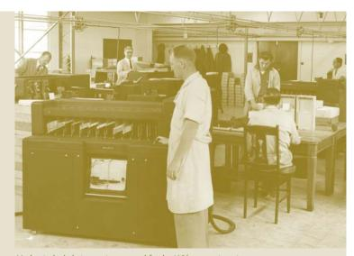
Mechanical tabulation equipment used for the 1954 census. A sorting machine is in the foreground.
